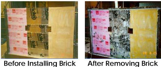
The test specimen consisted of a 12' wide by 8' high standard masonry cavity wall with three types of 2" thick insulation, extruded polystyrene (Figure 7, left sample), foil faced polyisocyanurate (center sample), and spray polyurethane (right sample).
