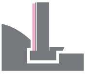
FOAMULAR® insulation is used to protect below grade waterproofing, even when insulating qualities are not needed. It is durable and light compared to asphalt board or other types of protective board often used. One person can place 4' x 8' sheets, saving time and labor.
