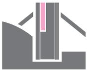
Some construction forming systems need void space inside the form. Durable and reusable FOAMULAR® insulation can be used to preserve such void spaces.
